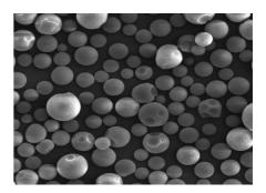
Zeochem extended its product range of bonded silica gels by new ZEObeads – amorphous porous silica gel as micro beads.
