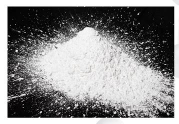
**ZEOflair 800** is a highly active, hydrophobic adsorbent for the removal of undesirable odors, flavors, and VOCs. Due to its three-dimensional open structure, ZEOflair 800 effectively removes odor/VOC molecules, including cyclic, highly branched, and some very polar compounds. This special adsorbent system can be easily incorporated as an additive to existing polymer formulations through a master batch or direct compounding.
